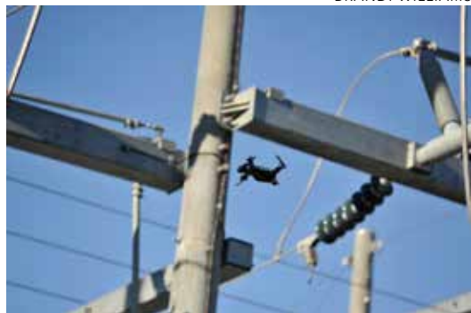
GETTING A CLOSE-UP: Drones fly very close to utility assets to take the clearest images and provide data to help co-ops keep an eye on how close vegetation is to equipment.
